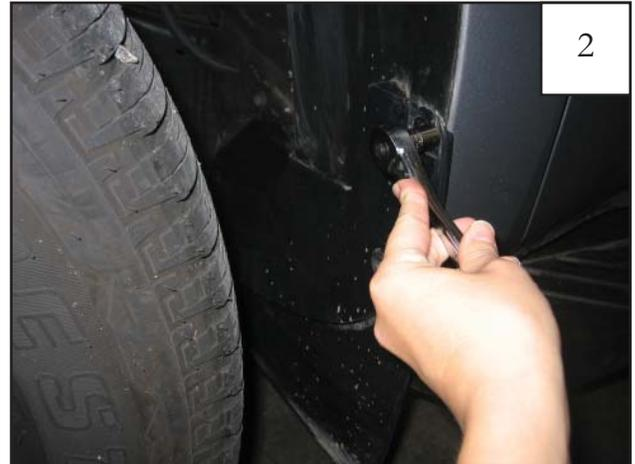
Using a socket wrench with a 10mm socket, remove top screw from factory mud guard as shown.
