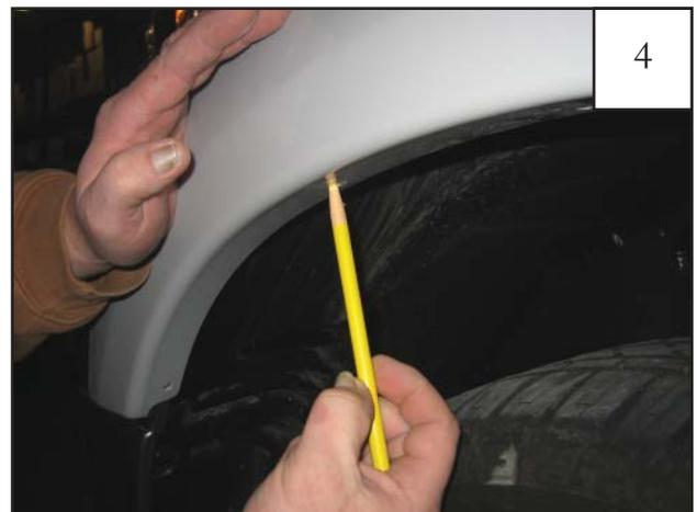
Hold the flare firmly on the fender. Starting with the second hole from the front of the flare, mark three clip locations with a grease pencil.
