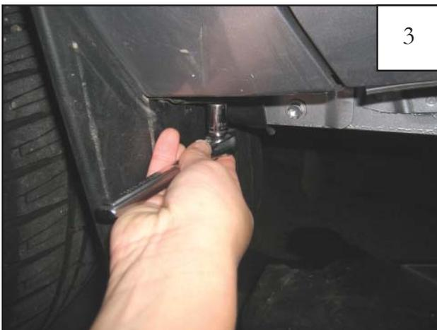
Remove screw from underside of factory mud guard. Note: If vehicle is equipped with running boards, running boards may need to be removed in order to access this screw.
